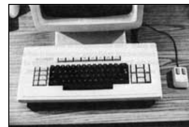
Figure 2. The Star keyboard and mouse. The keyboard has 24 easy-to-understand function keys. The mouse has two buttons on top
