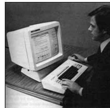
Figure 1. A Star workstation showing the processor, display, keyboard and mouse
